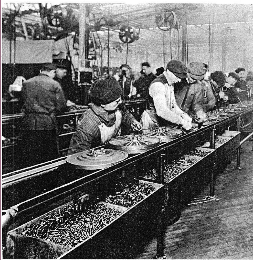
FIGURE 6.23. “The First Magneto Assembly Line,” 1913. This is a photograph of what Allan Nevins, among many other historians, called the first magneto assembly line. In his text, Nevins said that the magneto coil assembly was the first subassembly to be put on a line basis, but this illustration shows assembly of the flywheel magneto, the other half of the entire Model T magneto. (Henry Ford Museum, The Edison Institute. Neg. No. 833-167.)
